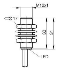
Inductive Sensors BES 516-329-G-E4-Y-03 M12x1 x 31 normally-open Sn=4mm shielded
